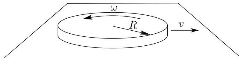
Note: It is important that the disk and the sliding surface (table, floor, carpet) should be perfectly level. Small friction is advantageous for the experiments (as the motion does not stop so fast). Sliding the disk on a carpet proved to be the best choice in my experiments.
